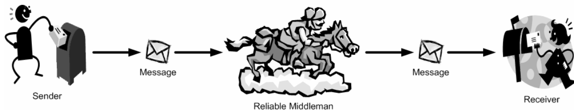
19 Figure 2.5: The Java EE “pony express” messaging model. Java EE adds reliability to messaging by adding a middleman that guarantees the delivery of messages despite network outages, even if the receiver is not present on the other end when the message is sent. In this sense, Java EE messaging has much more in common with the postal service than it does with common RPC protocols like RMI. We will discuss this model in much greater detail in Chapter 5.
