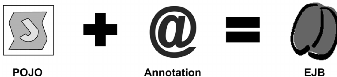
3 Figure 1.3: EJBs are regular Java objects configured using metadata annotations.
